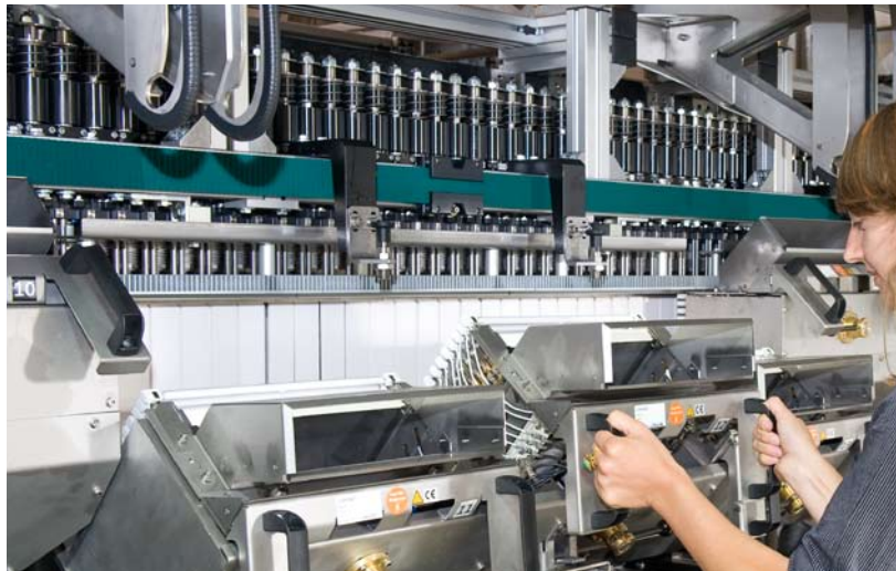
Light, compact and easily removeable heaters
