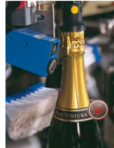
Mechanical container orientation using side-spotting bars (Photograph on the left)
