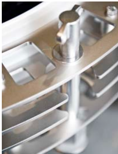
Guide starwheel with quick-lock (photograph at the top)
