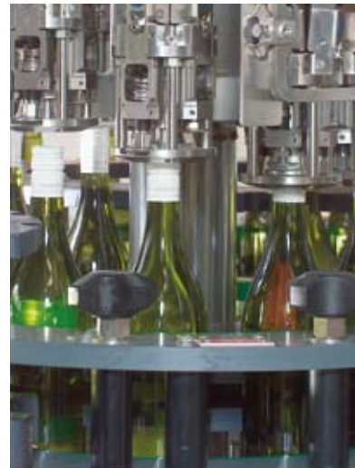
Rolling on of caps onto bottles
