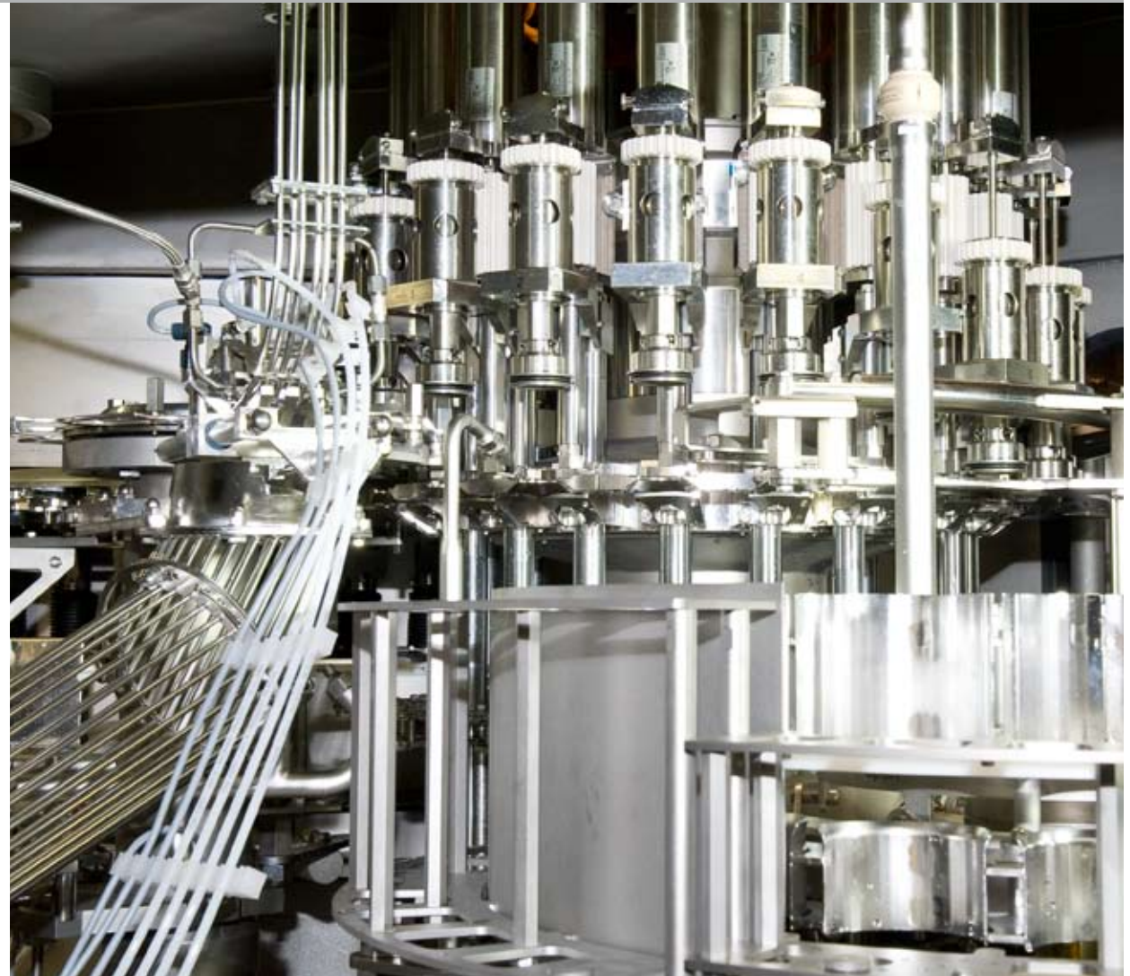
Cap feed chute with emptying device for cap change-over
