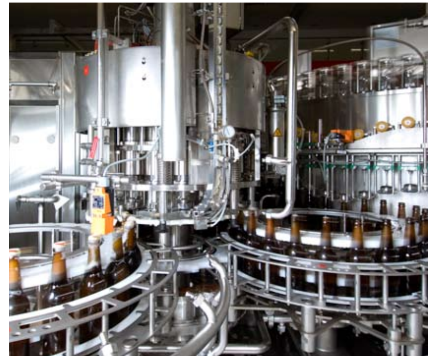
Crowner on the Sensometric VPVI filler
