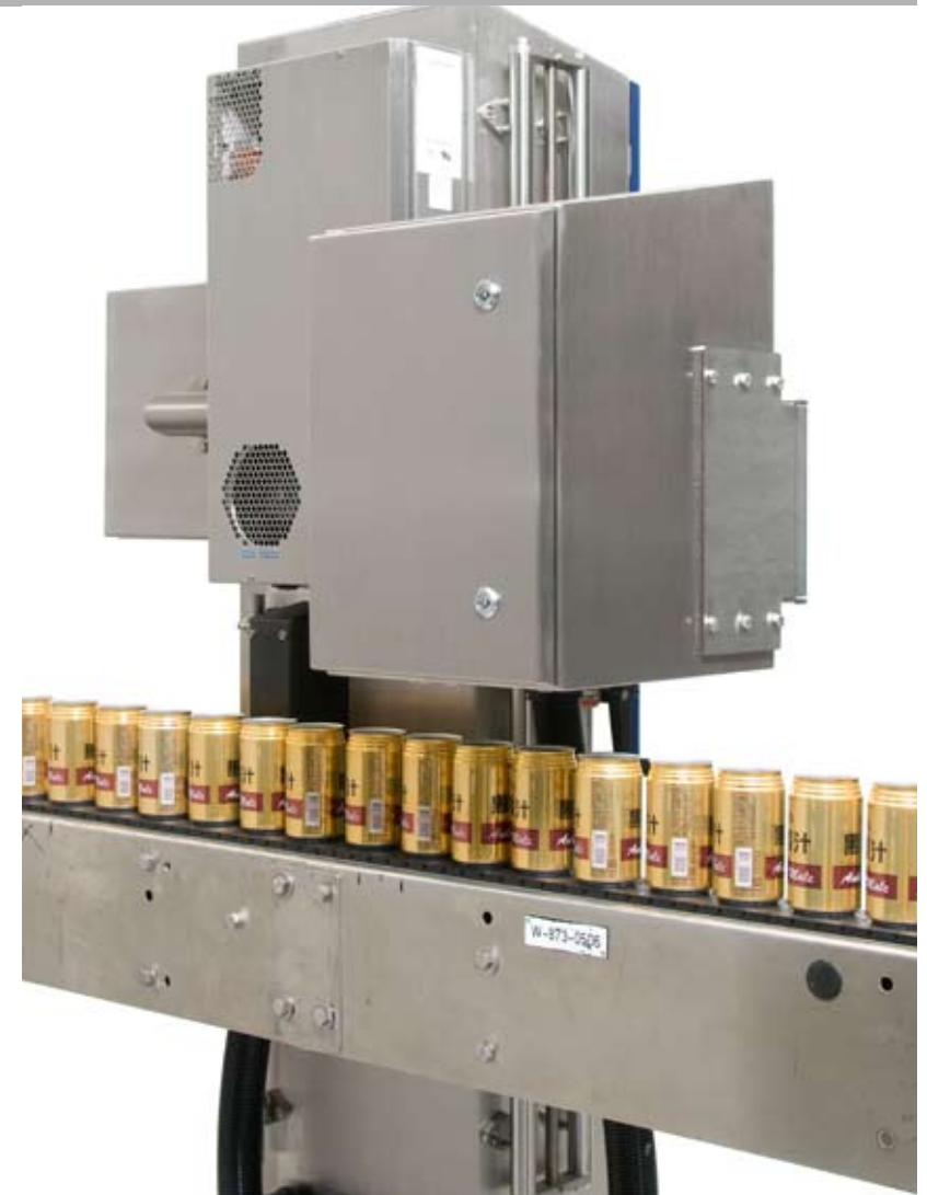
Camera unit and air conditioner
