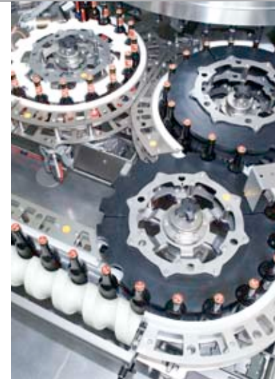
The Rapterc handling parts can be changed over easily
