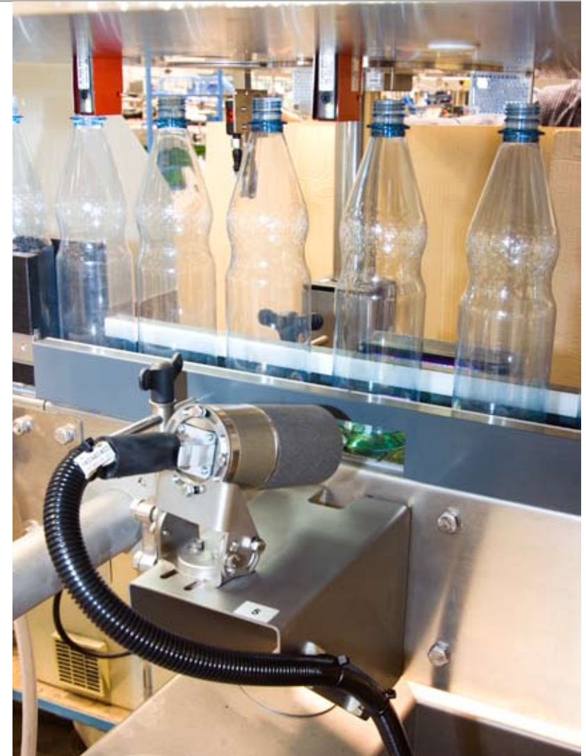
Liquid colour detection by camera
