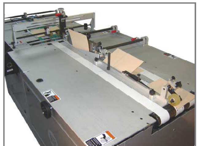
The folding section is aligned quickly and easily with the crease and performs the fold
