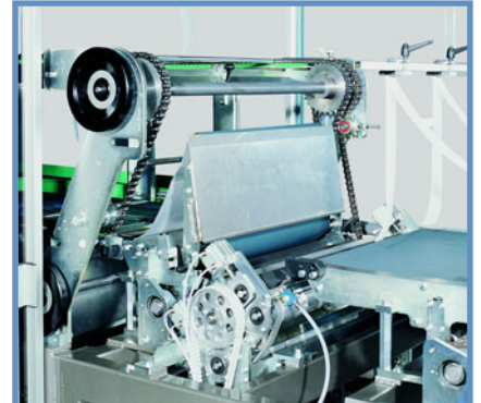
Film cutting unit New design has high precision during cutting phases for both neutral and printed films without the use of vacuum belts. Flip base allows for maximum accessibility for easy maintenance. Production up to 60 packages/minute based on product.
