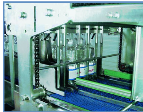
BASIC • Top pronged with alternating pneumatic movement, manually adjustable according to the required sizes • Production: up to 30 packages/minute based on product
