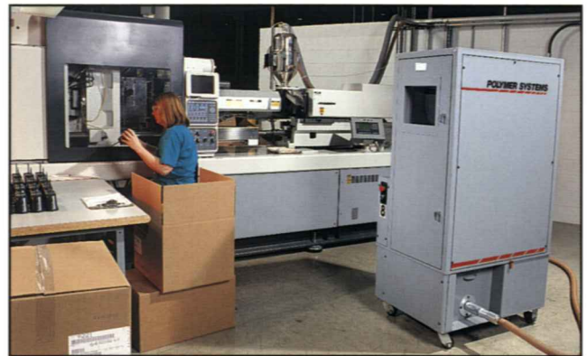
Vacuum bin under granulator evacuates regrind for blending with virgin resin in automated recovery system.
