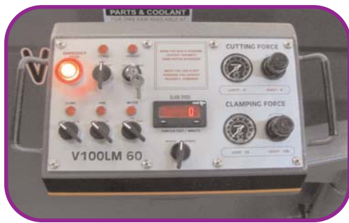
Console Pivots from Front to Right Side of Saw
