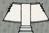
Figure 3 — Sanitary clamp end which can be utilized with a variety of quick-disconnect valves and fittings
