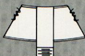
Figure 2 — I.P.S. Pipe size nipple which is adaptable to any pipe size fitting or valve.
