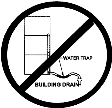
IMPROPER DRAIN LINE CONNECTION
