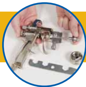
Remove the front cap and nozzle using a single tool
