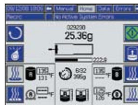
Recirc Mode option prevents materials from setting overnight
