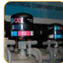
Desiccant Air Dryer
