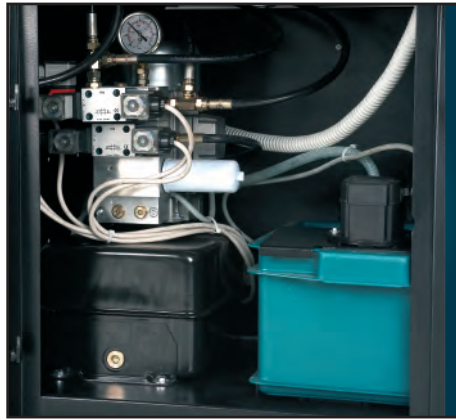
Hydraulic power unit and coolant tank included in the column
