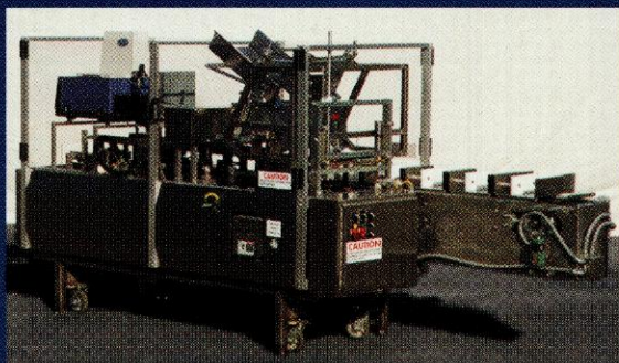
Bucketed Infeed Conveyor
