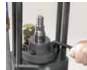
Packing gland is easily removed without special tools
