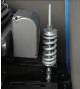
Automatic V-belt drive tensioning system.
