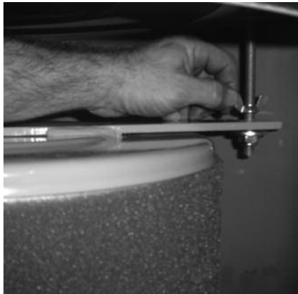
3. Loosen wing nuts, move them up about one inch.
