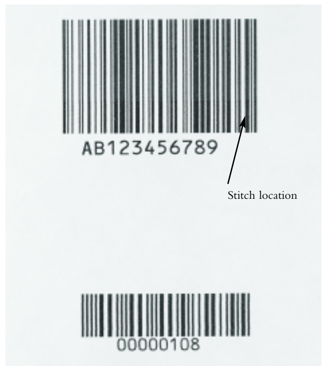
122mm (4.8") print swathe printed at 421 x 316dpi including electronic image stitching with two print heads
