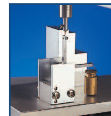
Automatic load cartridge calibration using traceable weights.
