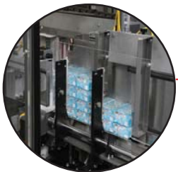
Progressive upstacking collates and stages product for loading
