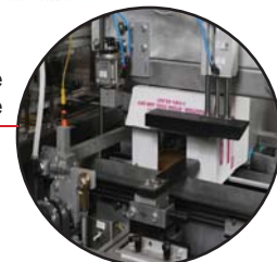
Horizontal Case Erecting and Discharge
