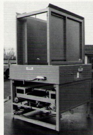
Automatic pallet dispenser. Factory set from 30" x 30" to 48" x 48". Capacity approximately 12 pallets.
