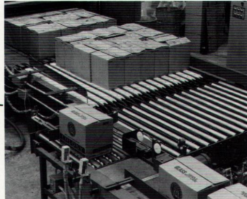
Heavy-duty dual chain arranging conveyor utilizes two drives, 60 pitch chains, 1/2" plate frame and accumulates one layer prior to the elevator.
