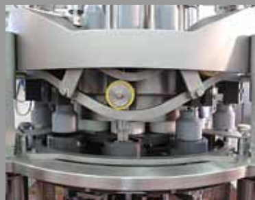
Single turret - product discharge area
