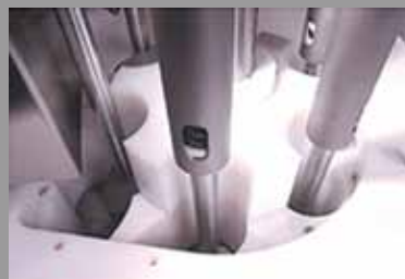
Dual turret "Slide Fill" style fill basin
