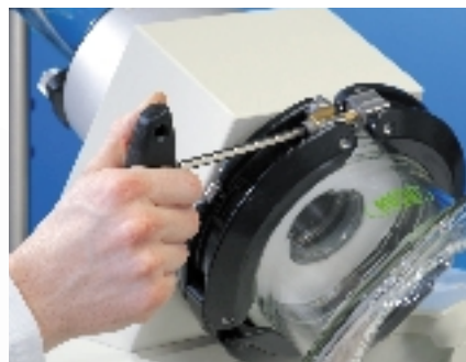
The evaporating flask is quickly and easily assembled with the innovative snap flange coupling and subsequently fixed securely by a turn wrench.
