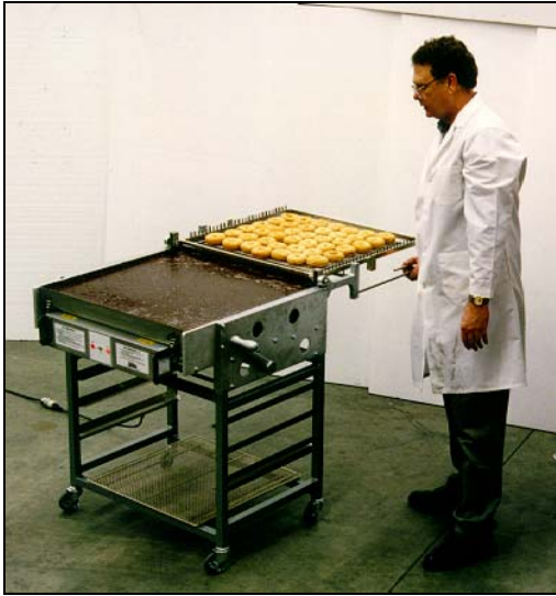
6. Rotate the wire / frame over the rack of donuts to be iced.
