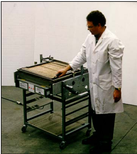
7. Firmly grip the two (2) handles and rotate the wire / frame and rack of donuts to be iced.
