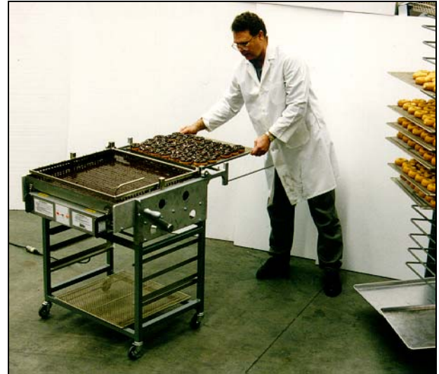
13. Rotate the wire / frame over the icing, remove iced donuts and repeat steps 1-13.
