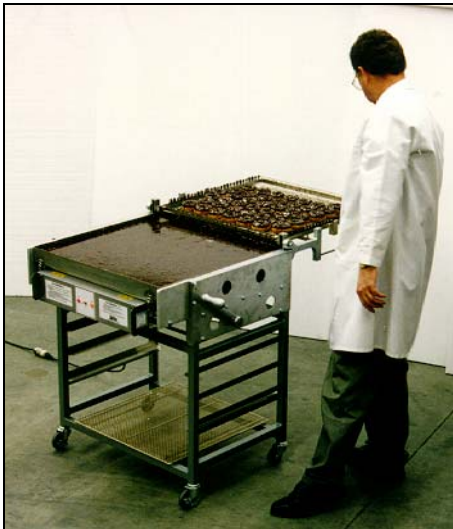
12. Firmly grip the two (2) handles and rotate the wire / frame and donut rack to the original position.
