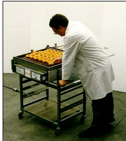
9. Push down on the icing lift handle to raise the icing pan until it reaches desired height.
