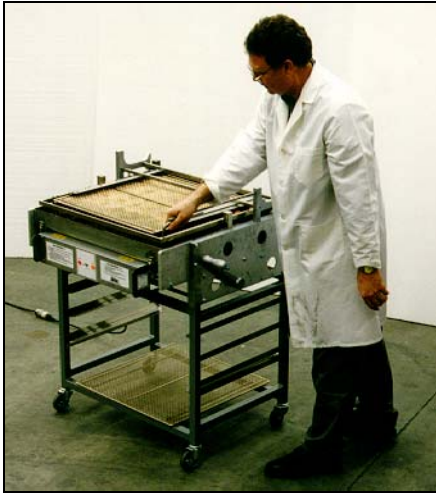
11. Rotate the empty donut rack over the iced donuts.
