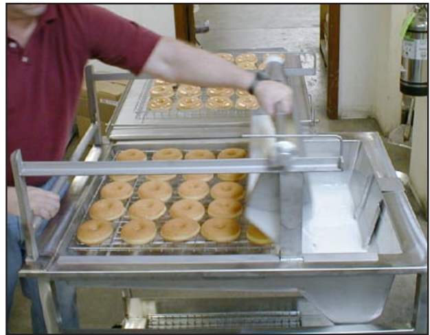
Above: EasyLift glazer in operation, showing sliding glaze applicator
