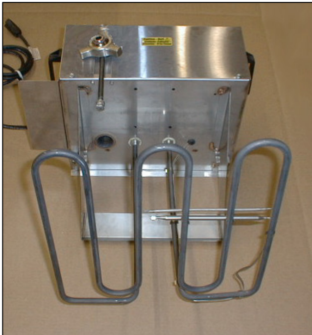
Figure 2-1. Removing the Heater Head. (Place heater head as shown above so no damage is done to the element.)
