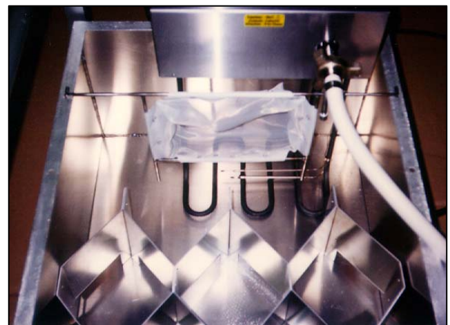
Figure 1-10. Positioning the Filter Frame for Melting.
