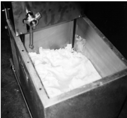
Figure 1-6. Packing Solid Shortening in the Kettle.
