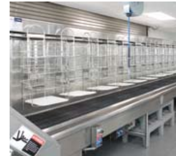
Cantilever design saves in labor costs
