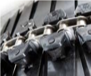
Slanted rollers allow for virtually frictionless belt operation
