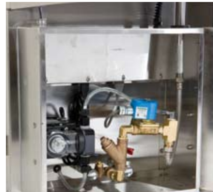
Belt wash cabinets where the cord is washed clean by spray jets
