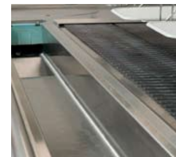
Built-in trough for scraps minimizes floor space
