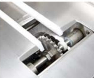
Sealed bearings require no lubrication
