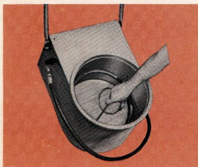
Hold-down ring is placed over filter paper.
