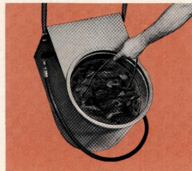
Remove sediment, sediment screen, and filter paper with special Anets tongs.
