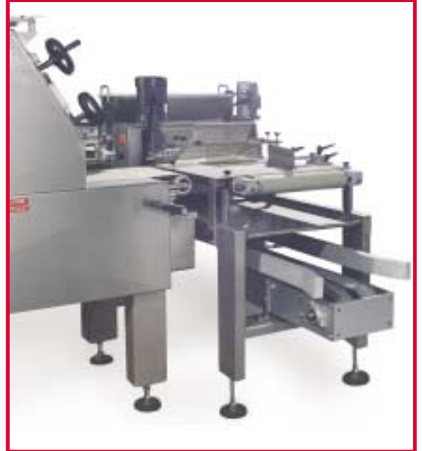
Easily removable endless transfer belt 18" wide. Delrin transfer plate and stainless steel adjustable plow. D.C. removable stainless steel rotary flour sifters.
