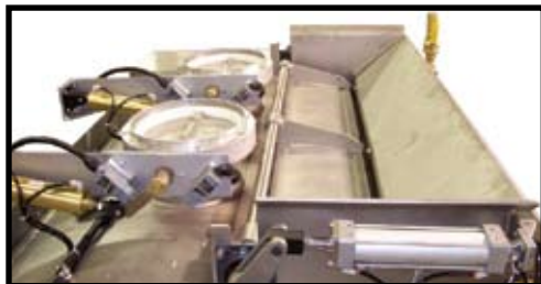
Mixer Top Canopy With Multiple Flour Inlets and Sponge Door
