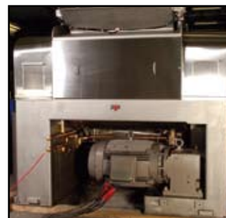
Rear Access Main Drive
