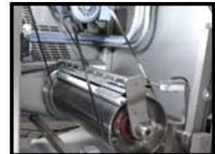
Cantilever Drum Design for Easy Blade Removal & Replacement
