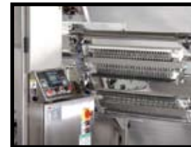
Self-Supporting Lattice Pull-out Mechanism
