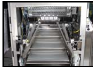
Extended Discharge Conveyor Guide Rails
