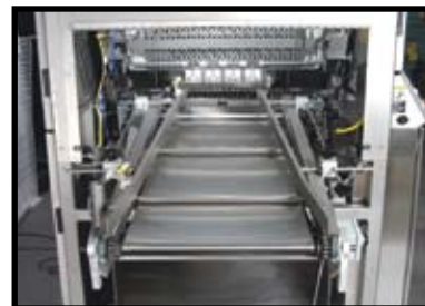
Extended Discharge Conveyor Guide Rails
