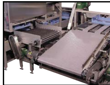
Discharge Conveyor with Kicker Conveyor
