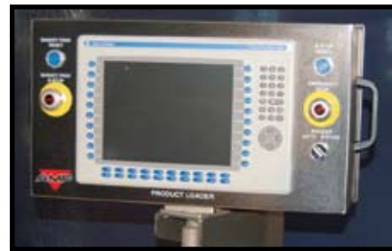
Operator Control Panel
