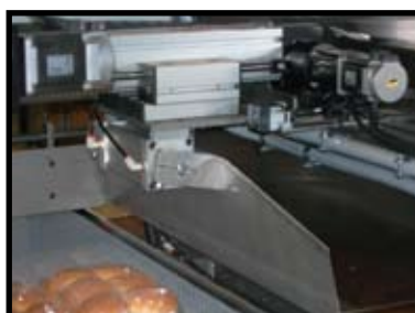
Smooth Servo Drives for Orienting Disk, Product Pusher, and Window Belt
