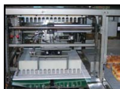
Smooth Servo Drives for Orienting Disk, Product Pusher, and Window Belt
