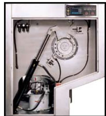
Hydraulic Tilt Mechanism Side With Special Operator Controls
