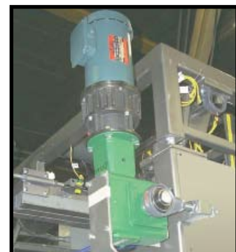
Main Carriage Drive
