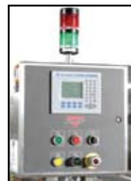
Operator Control Station
