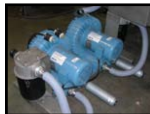
Easy Access, Cart Mounted Dual Vacuum Evacuation System
