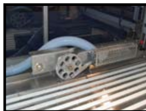
Advanced Hot Air Side Seal System
