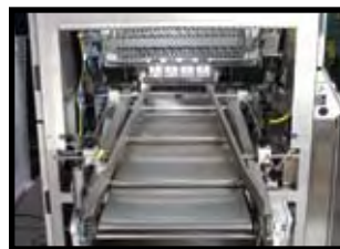
Extended Discharge Conveyor Guide Rails
