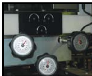
EZ Flow Manifold with Vane Adjustment Indicators
