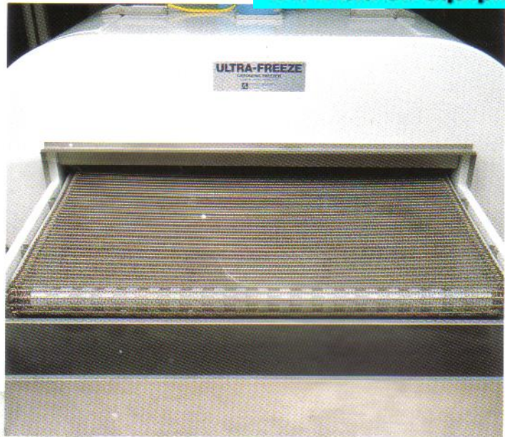
above: 48" Entry Vestibule with Standard Loading Cover Removed. Suitable for Hand Loading
