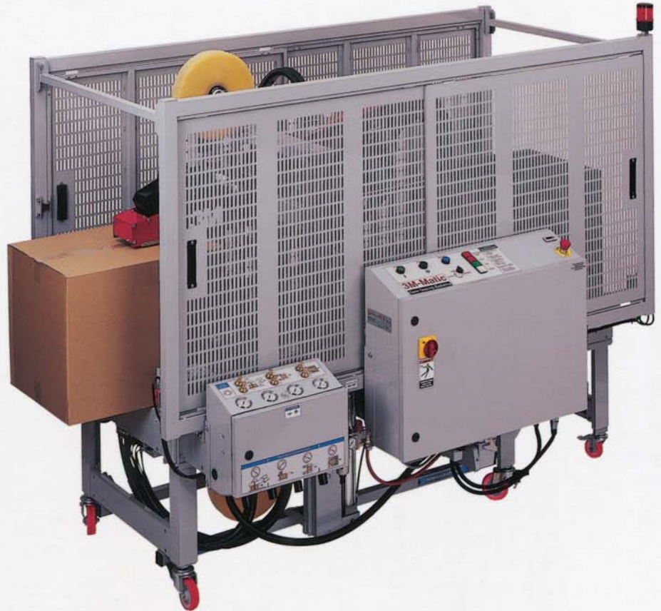
Perforated sheet metal shields allow visibility during operation and slide open for access. For safety, the 800rf will not operate with the shields open.
